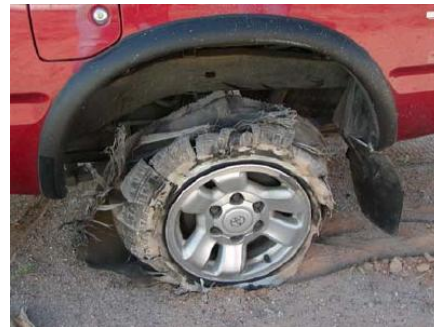
Sharp rocks, rebar, curbs
