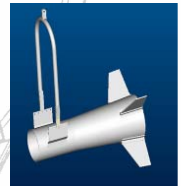
Acoustic Sweep: Generates Subsurface Acoustic Influence Field
