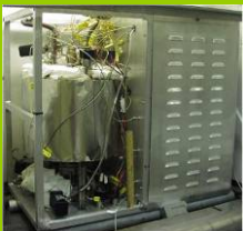
5kW Logistics Fuel Reformer (Regenerable S removable & CPOx reformer) GD / Aspen
