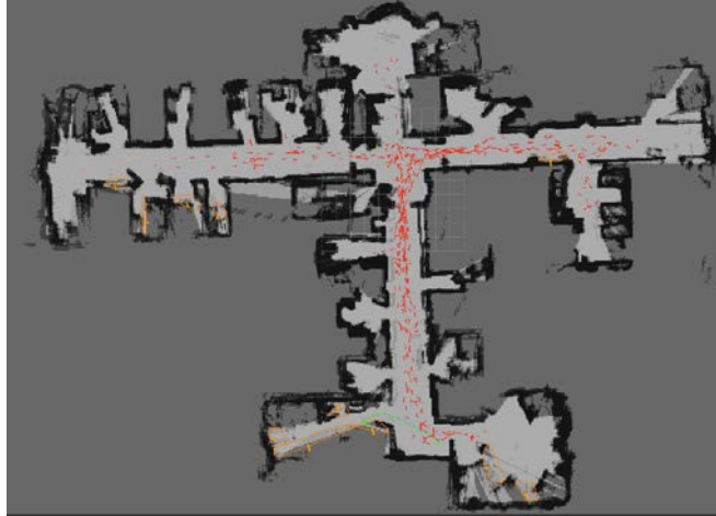
Fig. 7 Mapping of the second floor “hospital” building (abandoned children’s mental hospital), the urban rescue training facility
