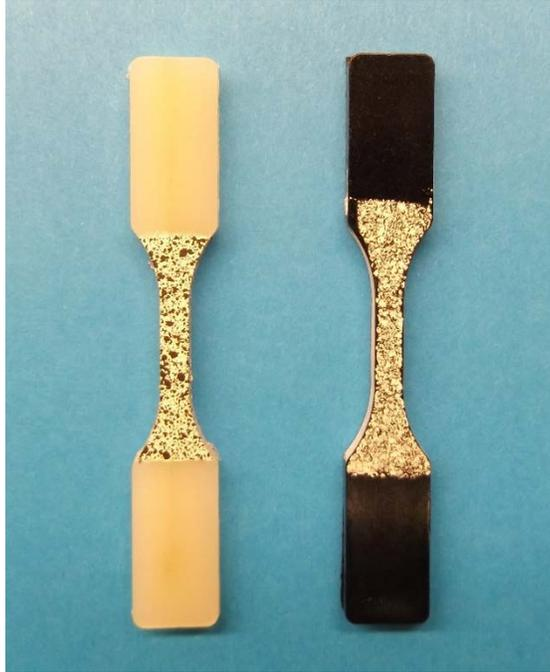
**Fig. 5** Injection-molded tensile specimens with DIC speckle pattern applied to gage section (0 wt% CER on left and 40.3 wt% CER on right)
