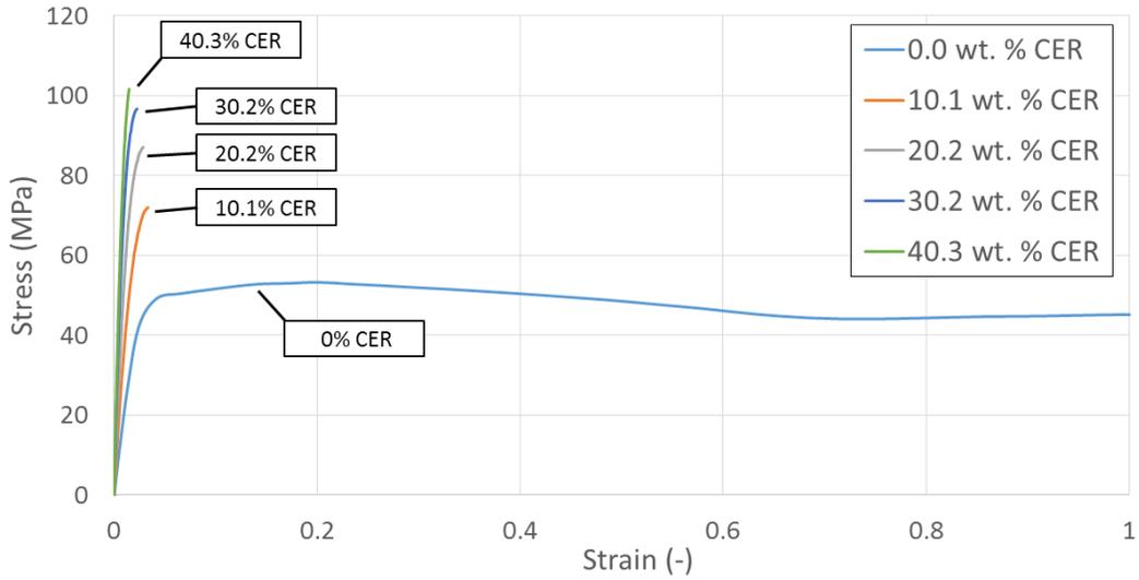
**Fig. 6 Tensile stress-strain relation for the 5 compositions of CER/nylon**
