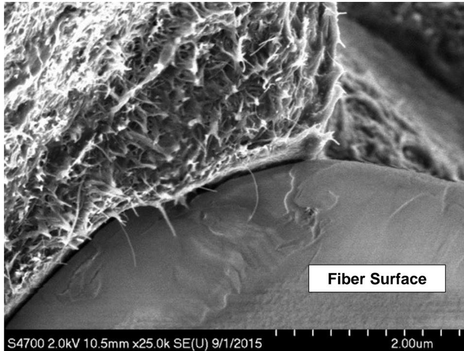
**Fig. 11** Close-up SEM image of glass fiber–nylon matrix interface in 100 wt% CER test specimen
