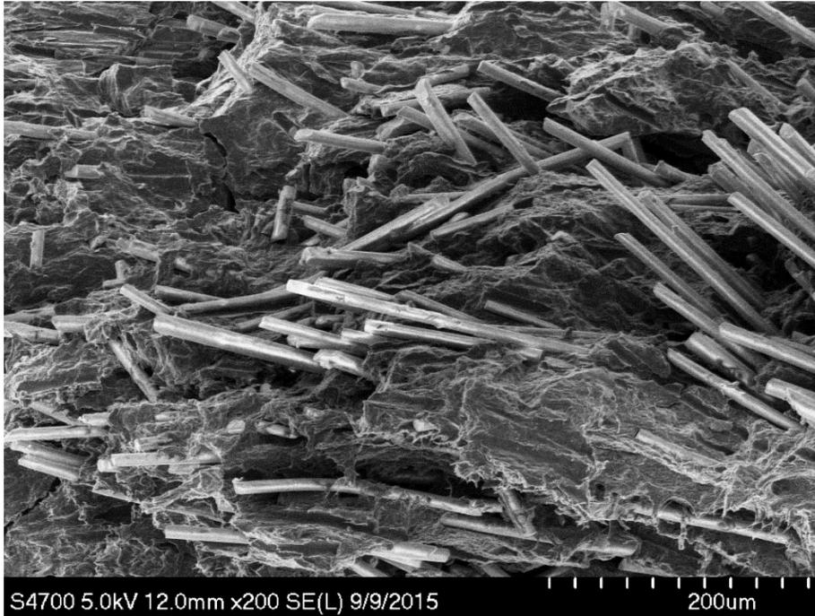
**Fig. 4 SEM image of CER pellet fracture surface**
