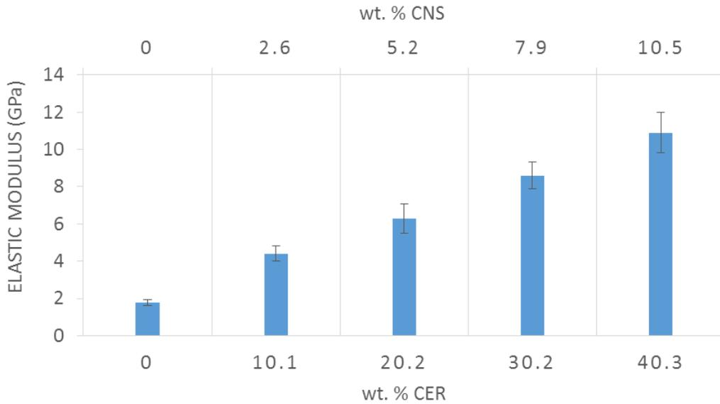
**Fig. 7 Average and standard deviation in elastic modulus as a function of composition**
