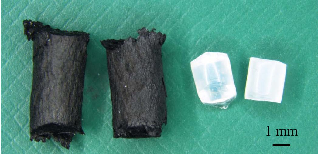
**Fig. 2** As-received CER pellets (left) and neat nylon pellets (right)
