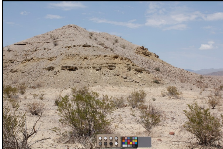
Figure 4. Calibration standards setup for visible acquisition.
