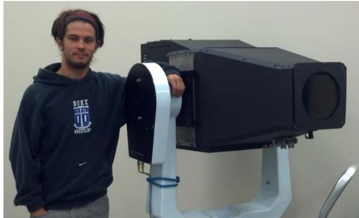
AWARE 2 folded camera, 40 \mu rad IFOV, 50° by 30° FOV, fits in a commercial airline carry-on bag.
