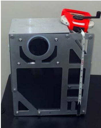
AWARE 2 folded camera, 40 \mu rad IFOV, 50° by 30° FOV, fits in a commercial airline carry-on bag.
