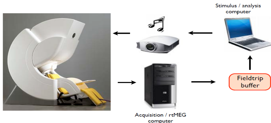
Figure 3.3 Illustration of a typical setup with rtMEG. The Acquisition computer controls the acquisition, stores the data and runs the rtMEG interface. Another computer drives the experimental paradigm by providing stimuli to the subject and sending trigger events that eventually go to the MEG data file. The rtMEG interface writes data to the Fieldtrip buffer, which can be run by rtMEG or by any other computer in the network. The application(s) reading from this buffer can run on the stimulus computer or on any other computer connected in the network.
