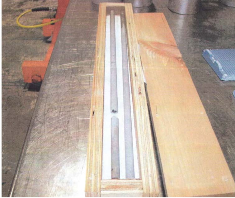
Fig. A-2 Cold-sprayed Biodur tubes after unpacking at Solar Atmospheres. One of the tubes has been cracked, forming 2 pieces.
