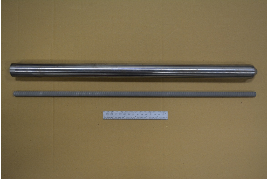
Fig. 1 Picture of a Stellite 25 liner and a steel barrel blank. The liner has been sprayed with a thin layer of tungsten carbide particles.
