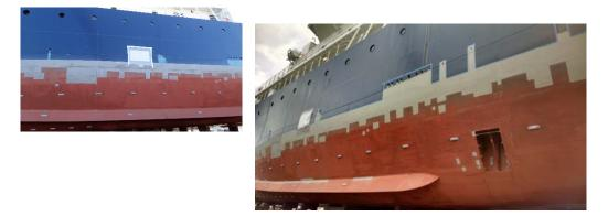
• Hull Coating – DCI is making repairs to the paint system above the water line as needed.
