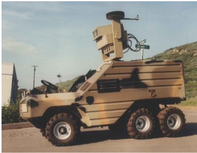
Figure 154. a) The STV turns west off Woodward onto Robart Road during onsite testing in San Diego, CA. b) Shown here with its RSTA Module partially elevated, the STV was controlled by a motorcycle-type steering device (inset lower right) on the operator control unit (image courtesy General Dynamics Robotic Systems).
