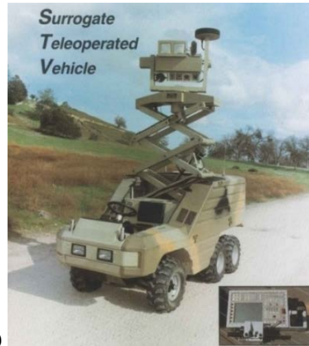
Figure 154. a) The STV turns west off Woodward onto Robart Road during onsite testing in San Diego, CA. b) Shown here with its RSTA Module partially elevated, the STV was controlled by a motorcycle-type steering device (inset lower right) on the operator control unit (image courtesy General Dynamics Robotic Systems).
