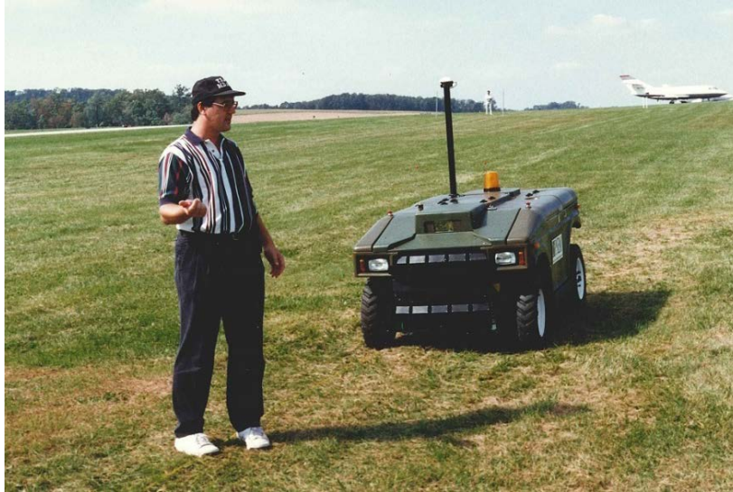
Figure 202. RST vice president Mark Del Giorno evaluates early autonomous GPS-based route execution at the company's Westminster facilities prior to the addition of collision avoidance, circa 1996.
