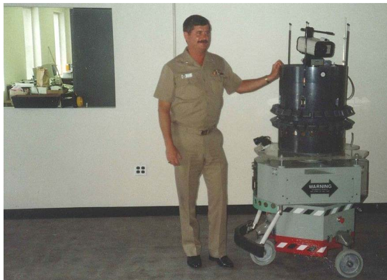
Figure 144. Shown here atop a Cybermotion K-2A Navmaster mobility base, the ARDEC MDARS-Interior payload was a 24-inch-diameter ModBot configuration with six stacked modules for video, acoustic, microwave, passive infrared, sonar, and security assessment.
