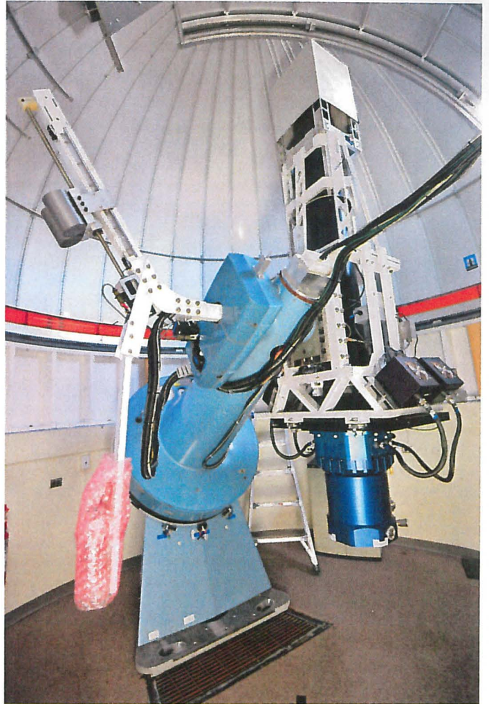
The USNO Robotic Astrometric Telescope. The white top box serves as dust protection and contains the motorized lens cover (206-mm entrance pupil aperture). The blue dewar contains four big CCDs (111 million pixels each) and has a 300 mm dewar window that also serves as the bandpass filter. Note the moving counterweight on the left arm, which is needed to balance the changing weight of LN 2 fill of the dewar. (Image credit: Norbert Zacharias/USNO.)
