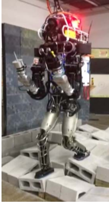
Figure 72. Atlas at a Joint Limit when Descending Cinderblocks
