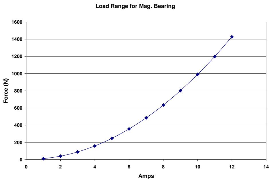
Fig. 11. Graph illustrating the amount of load that the magnetic bearing can apply to the rotor.
