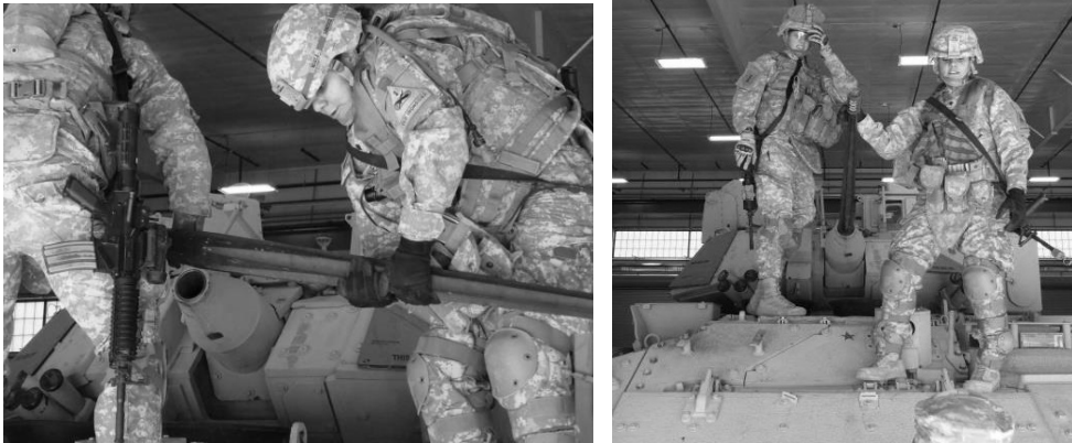
Figure 1.5. Image of Soldiers Installing the Barrel of the 25mm Gun on a BFV (Task 5)
