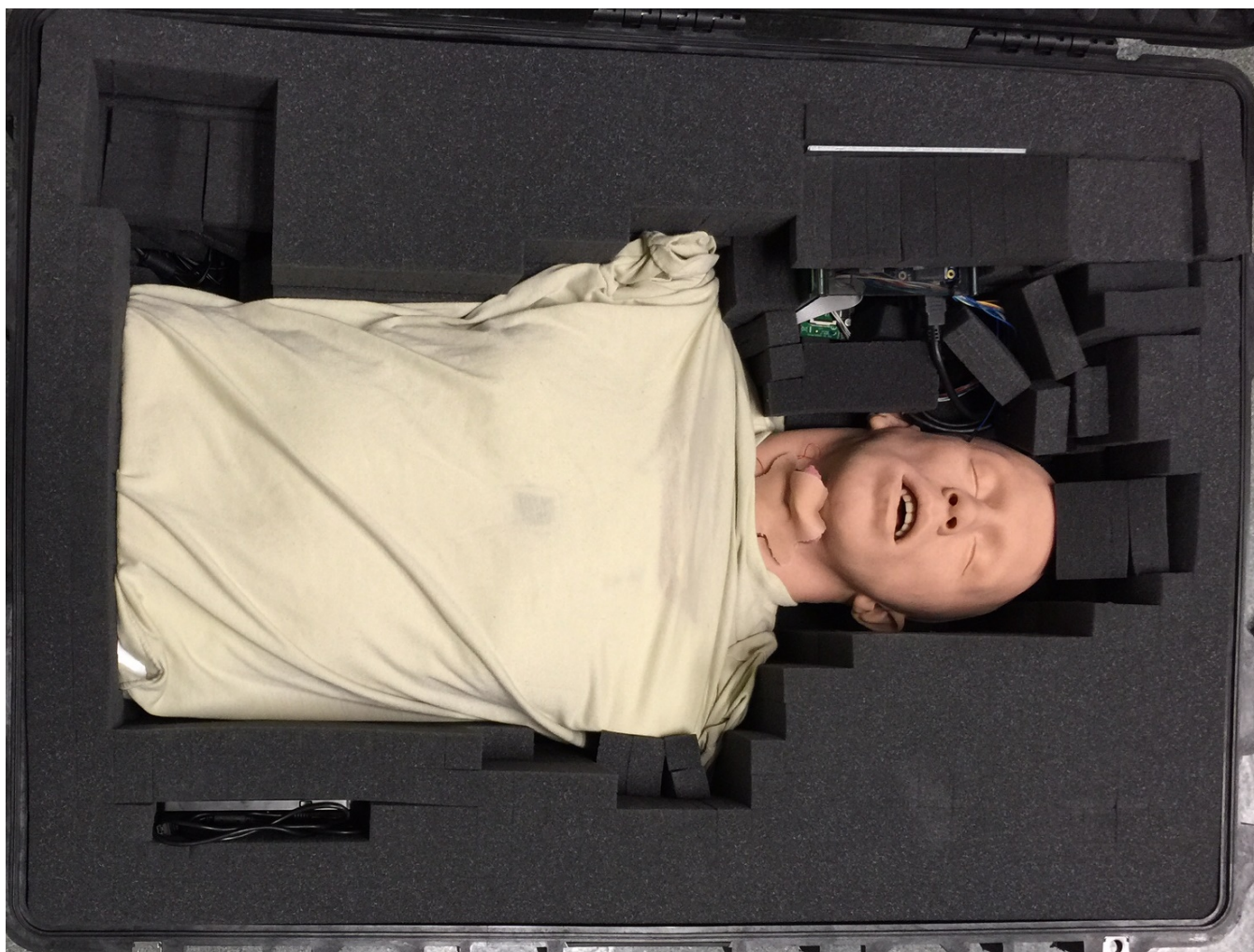
Figure 5: Airway Model with sensors, computer, key board and power supply ready for shipping.
