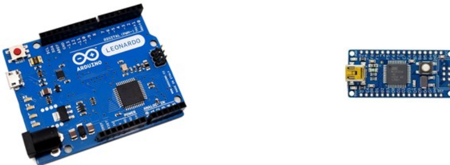
Figure 14a and b: Large and Small Arduino brand micro controller with USB interface
