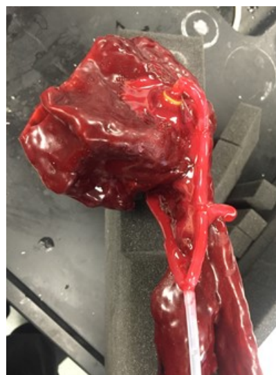
Figure 30: Plumbing embedded within model for testing
