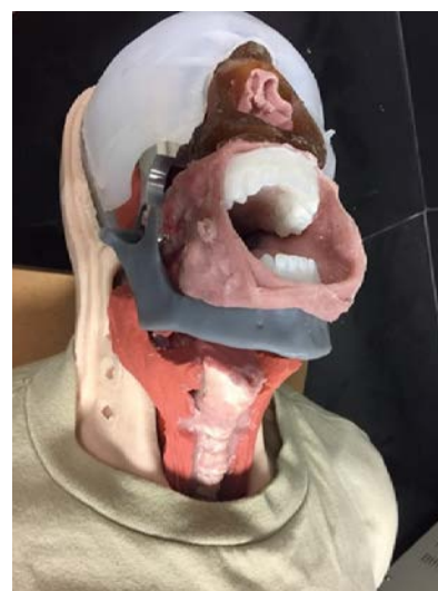
Figure 34: shows an inner-view of a model with embedded sensor, ducts, connectors, plumbing, and wiring, integrated into 7 Sigma head and torso.
