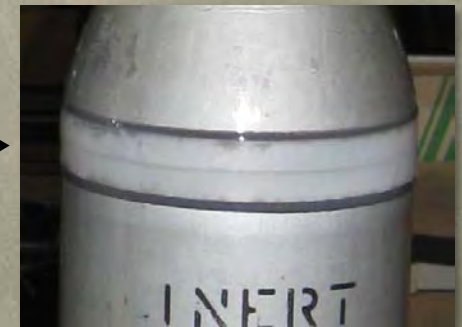
Polypropylene Band Edges Sealed with epoxy
