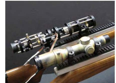
Figure 0. Barrel position sensor and reticle compensation system.
