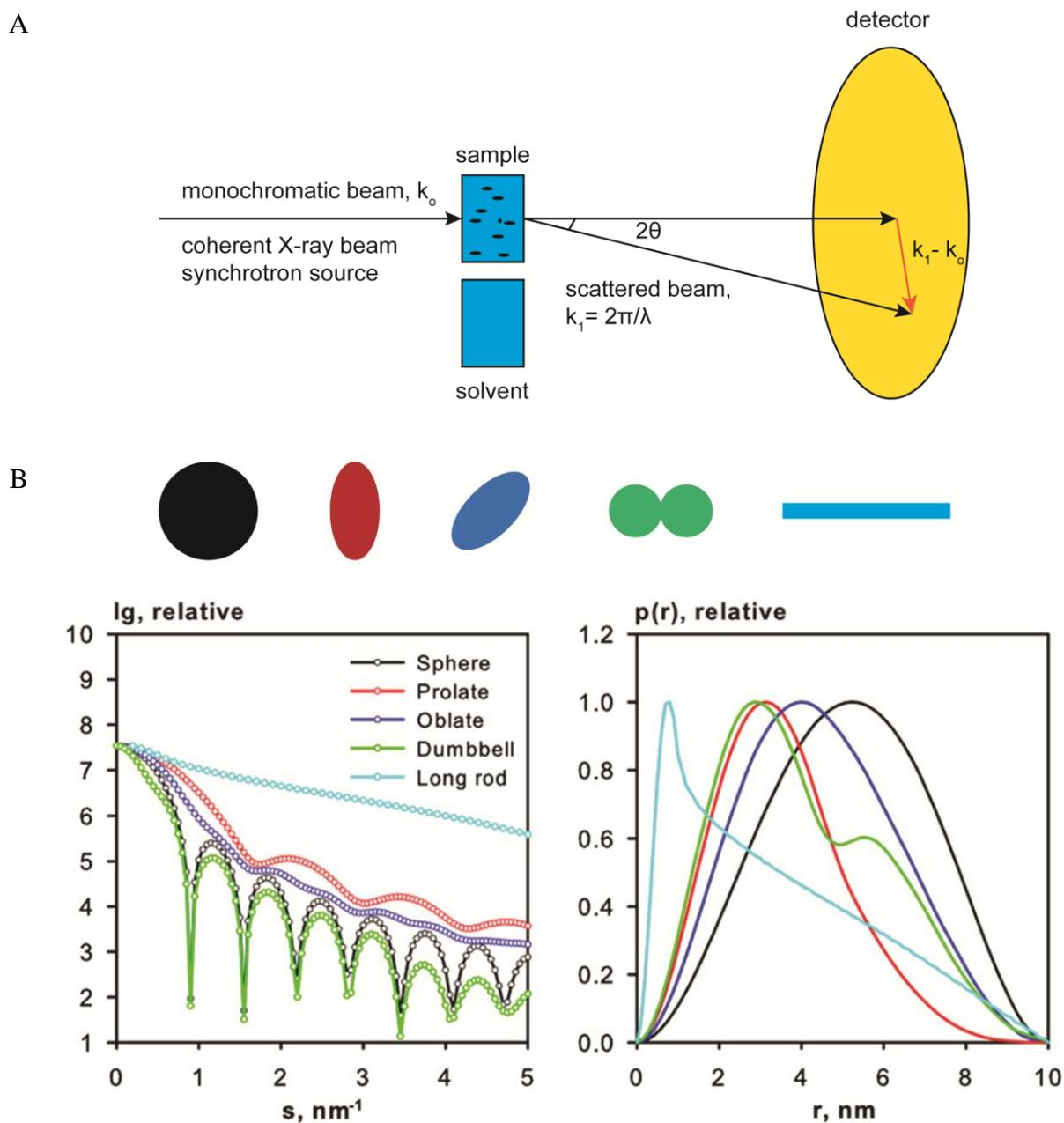
**Figure 2.4** (A) Schematic representation of small angle X-ray scattering. Adapted from Mertens and Svergun 2010. (B) Scattering intensities and distance distribution functions,  $P(r)$  calculated for typical geometric shapes. Solid shapes (black), prolate ellipsoid (red), oblate ellipsoid (blue), two domain (green) and long rod (cyan). Diagram taken from Mertens and Svergun, 2010.
