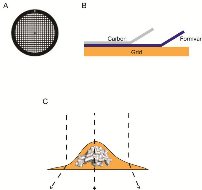
**Figure 2.5/** Diagram showing components used in negative stain transmission electron microscopy. (A) Copper grid 200 mesh square. (B) Transverse section of grid showing carbon and formvar layers. (C) Electron scattering through protein sample stained with heavy metal salts.
