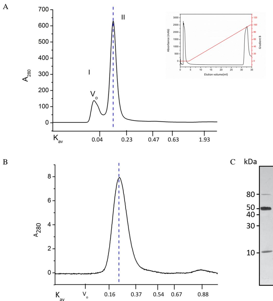
**Figure 5.6** SEC chromatograph of  $[H_6Lsm\alpha]_7$ . (A) Preparative grade SEC (Superdex 200 16/600) column pre-equilibrated with 20 mM Tris pH 8.0, 150 mM NaCl, 2% glycerol with a flow rate of 1 mL/min. IMAC elution profile provided in inset. (B) Analytical SEC (Superdex 200 10/300) column, in the same buffer as above with a flow rate of 0.4 mL/min. (C) SDS-PAGE of purified  $[H_6Lsm\alpha]_7$ .
