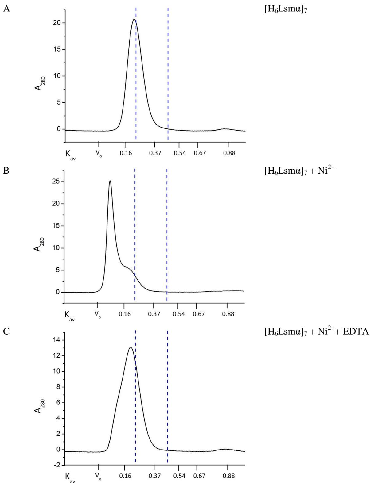
**Figure 5.14** SEC traces showing solution behaviour of  $[H_6Lsm\alpha]_7$  on addition of  $Ni^{2+}$  (0.2 mM). The dotted lines represent elution position of  $[H_6Lsm\alpha]_7$  complex and single-ring form. The running buffer was 20 mM Tris, pH 8.0, 150 mM NaCl, 2% glycerol. Sizing column used was a Superdex 200 10/300 column run at a flow rate of 0.4 mL/min.
