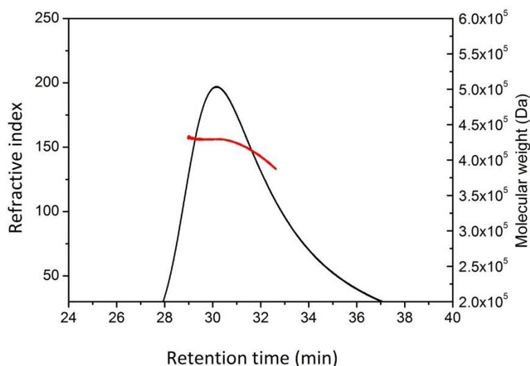
**Figure 5.10** | Static light scattering showing the molecular weight distribution of  $[H_6Lsm\alpha]_7$ . The run was operated in 20 mM Tris, pH 8.0, 150 mM NaCl, 2% glycerol at a flow rate of 0.4 mL/min.
