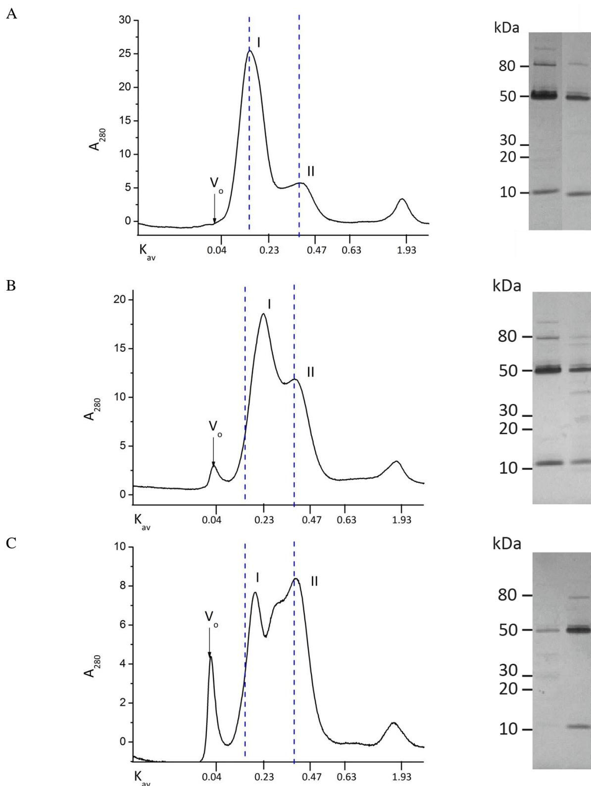
**Figure 5.12** SEC profiles of  $[H_6Lsm\alpha]_7$  in presence of EDTA carried out in Superdex 200 16/600 with a flow rate of 1 mL/min. (A) 10 mM EDTA, 4 h. (B) 15 mM EDTA, 24 h. (C) 15 mM EDTA, 48 h. Dashed lines indicate position of the  $[H_6Lsm\alpha]_7$  complex and single ring.
