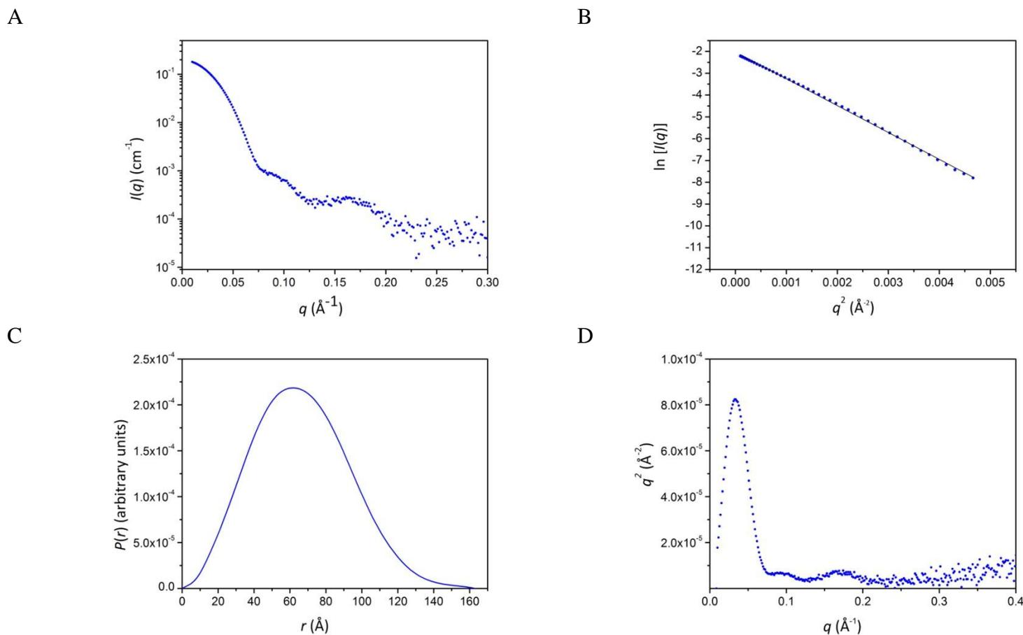
**Figure 5.15** | SAXS data recorded at SAXS/WAXS beamline at Australian Synchrotron. The following parameters were calculated for  $[H_6Lsm\alpha]_7$  loaded onto the SEC column at 2 mg/mL (A) Scattering curve. (B) Guinier approximation. (C) Distance distribution function. (D) Kratky representation of scattering data.
