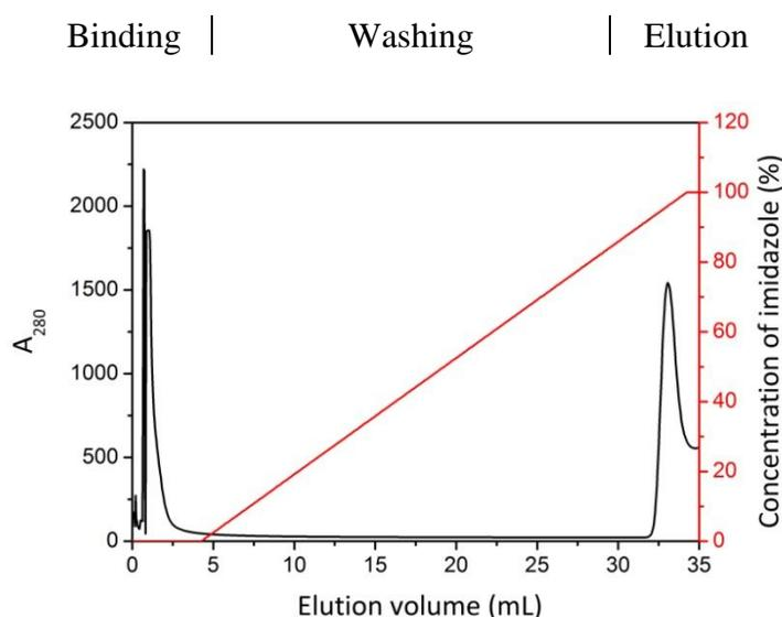
**Figure 2.1** | Typical trace of immobilised metal affinity chromatography. The binding, washing and elution steps are shown above the graph. Absorbance at 280 nm (mAU) is shown in black and concentration of imidazole is in red.
