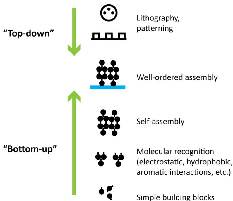
**Figure 1.1|** A comparison of the “top-down” and “bottom-up” approaches applied to manufacturing of nanomaterials. The “bottom-up” approach is based on the interactions of simple building blocks which can self-assemble into well-ordered complex structures. Schematic adapted from Gazit (2007) <sup>12</sup>.
