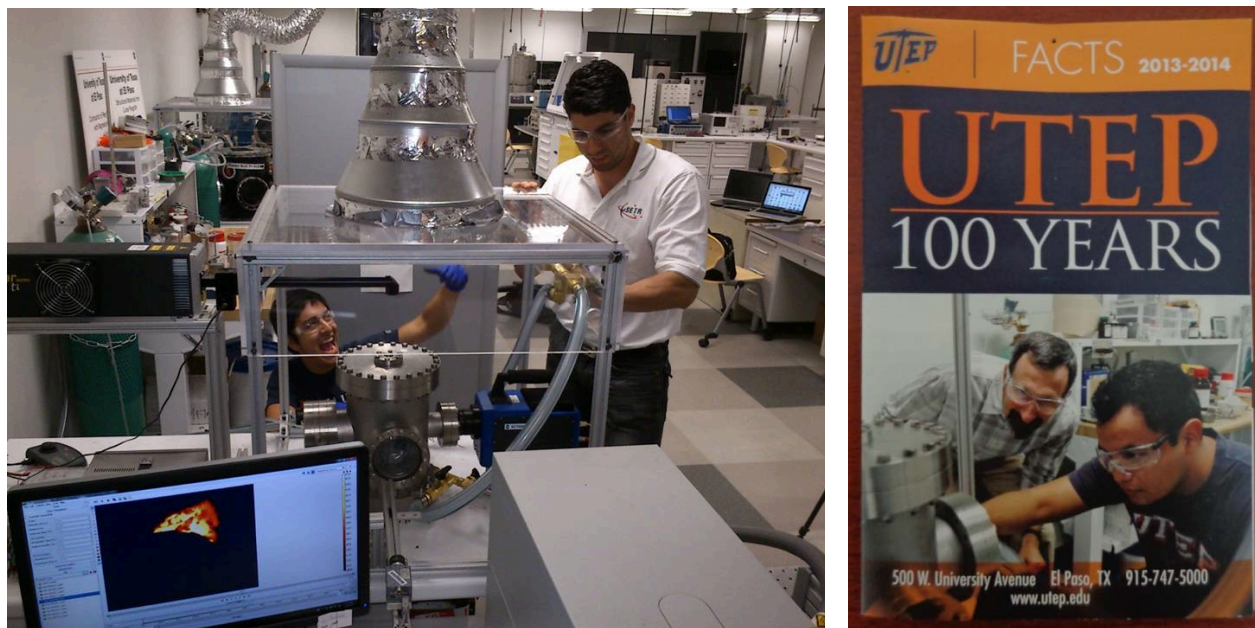
Figure 1. UTEP students Marco Machado (left), Daniel Rodriguez, and Sergio Guerrero (right picture) are working with an experimental setup for laser ignition of gas-generating mixtures.
