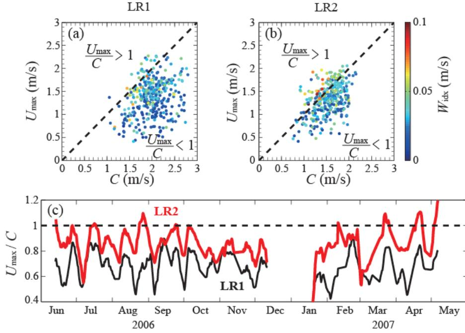
Figure 4. Scatter plots between maximum current velocity,  $U_{\max}$ , and propagation speed  $C$  of ISWs observed at two mooring sites, (a) LR1 and (b) LR2.  $W_{idx}$  is the vertical speed averaged during the wave period. Panel (c) shows the temporal variation of the convective instability condition at LR1 and LR2. The dashed lines indicate  $U_{\max}/C = 1$ .
