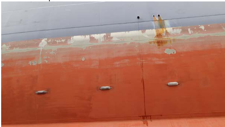
Example of Port Side AF Failure
