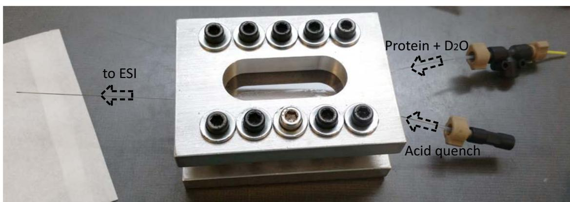
**Figure 8.3** The assembled microfluidic chip for site-specific hydrogen-deuterium exchange experiments. The capillary-based protein-deuterium rapid mixing device (Figure 8.1) was integrated onto the microfluidic chip (Figure 8.2) for localised analysis. The input and output capillaries are labelled.
