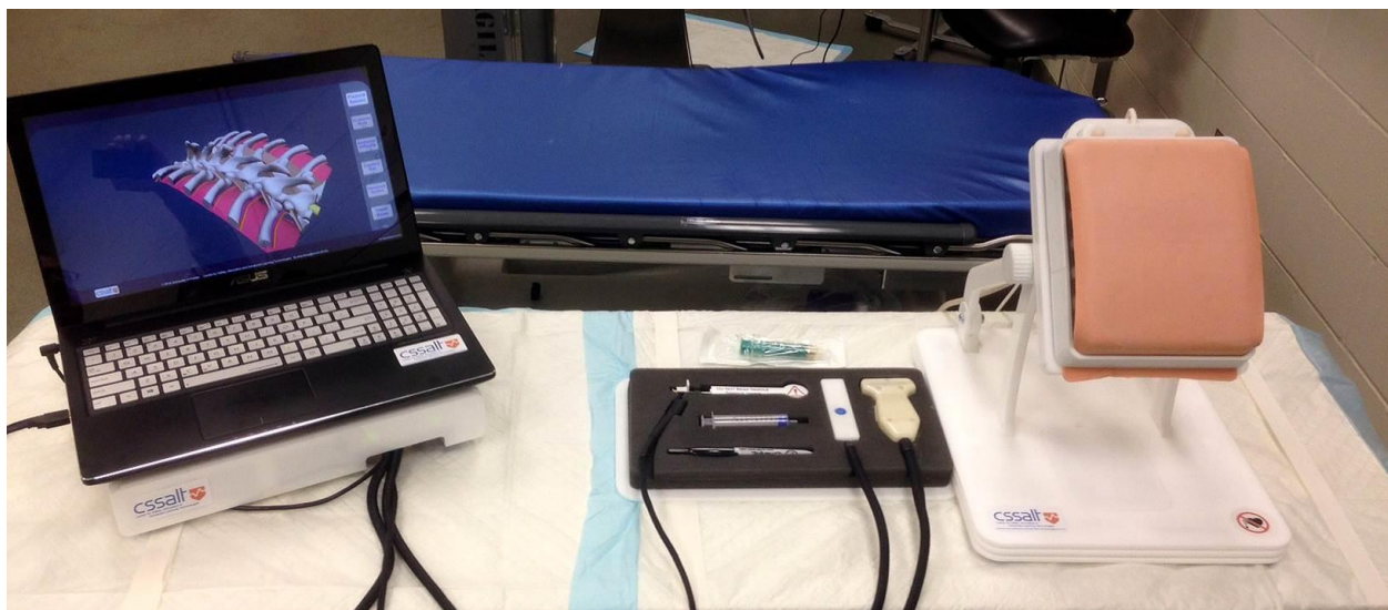
Figure 1. The modular stand is on the right of the photo. It is shown in the thoracic regional anesthesia simulator configuration, i.e., with an RA anatomical module representing the posterior upper thorax snapped and indexed into the modular stand. Thoracic paravertebral blocks (TPVBs) and other regional
