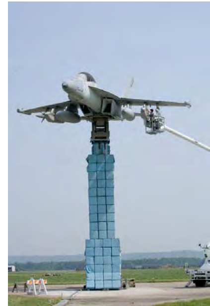
Antenna Pattern Testing
