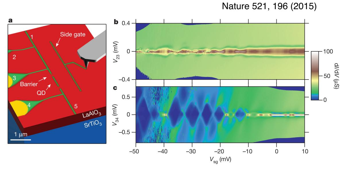
schematic of device demonstration of single-electron transistor behavior in the sketch-FET, and the negative-U model describes the filling. The negative-U is sufficient to pair the electrons on the nanoscale
