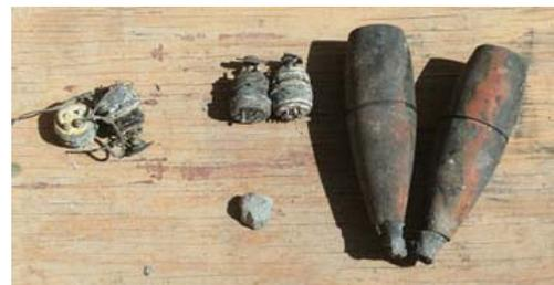
OEF IED attack on a MRAP carrying 16 60mm High Explosive M768 Mortar Cartridges. The IM design features resulted in the fuze separating from the shell body preventing high order detonations thus saving the lives of the Soldiers.
