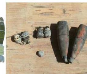
Shell bodies and separated M768 cartridges recovered from the vehicle after the fire.
