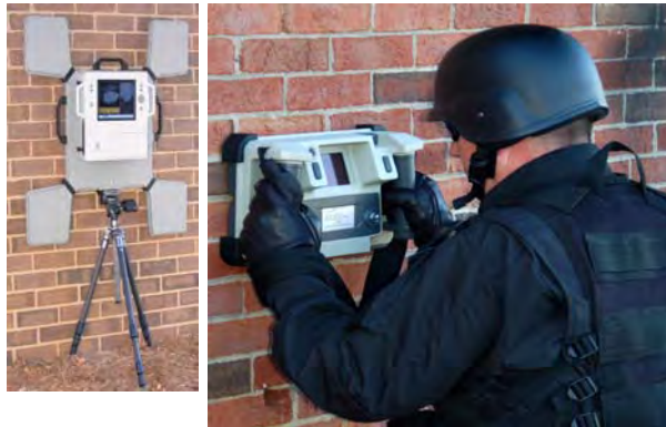
X800/X400 Through-Wall Imaging
