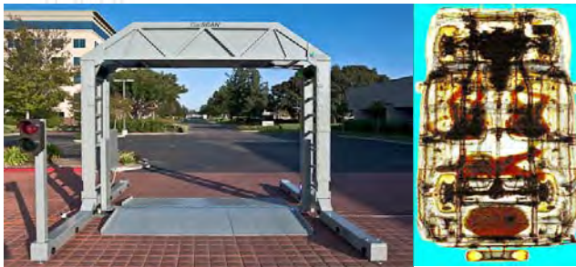
Car Scan – Dual Energy Low Dose X-Ray
