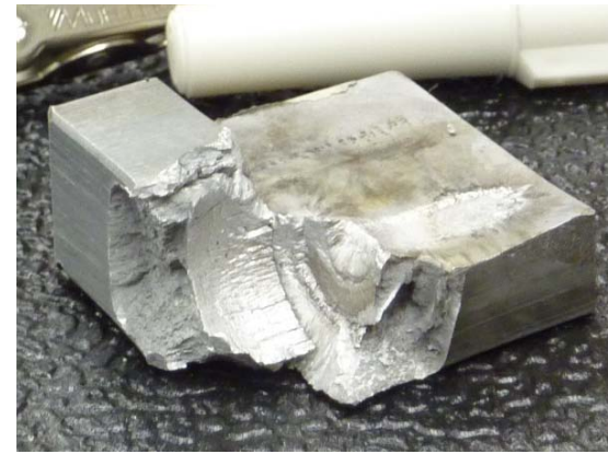
Dent Block After Successful Charge Transfer
