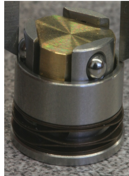
Only under All- Fire does the locking sleeve unlock the striker.
