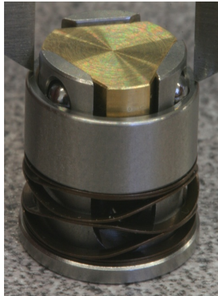
Under No-Fire acceleration locking sleeve will return back to equilibrium
