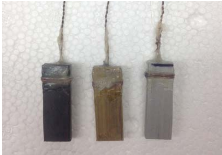
Figure 14. Original coupon construction (from left to right): A36 steel, brass, and aluminum with attached copper wire sealed in epoxy
