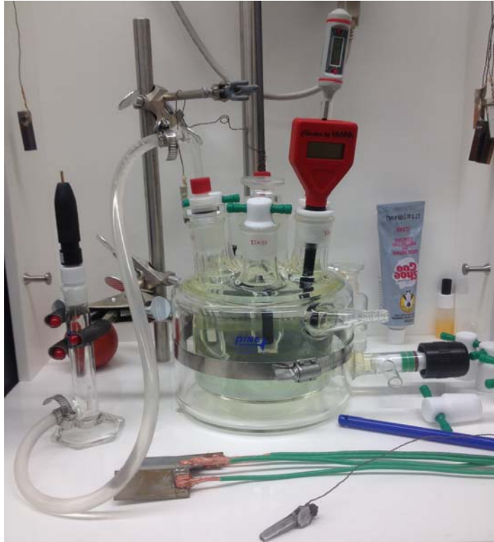
Figure 15. Pine Instruments 3-electrode 1L corrosion cell.
