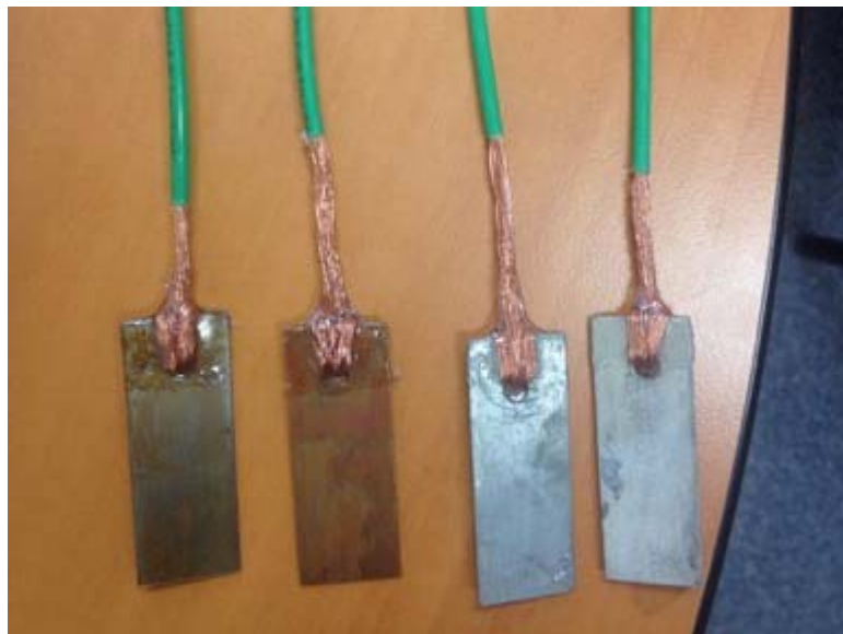
Figure 8. Electrochemical experiment coupon set-up.
