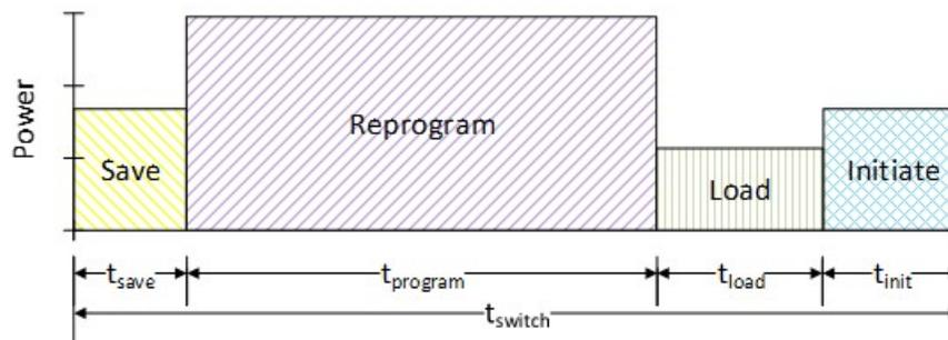
**Figure 15: Example of a Context Switch Timeline**
