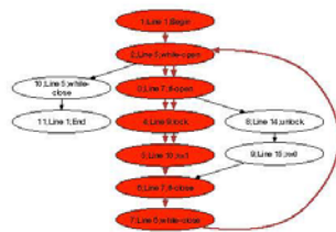
Figure 5. This is the CFG corresponding to the lock/unlock while loop code.
