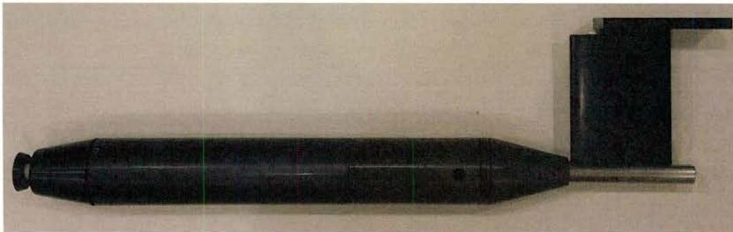
Fig. 1. The vehicle model with the enclosed ZNMF thruster. The orifice is near the aft section.
