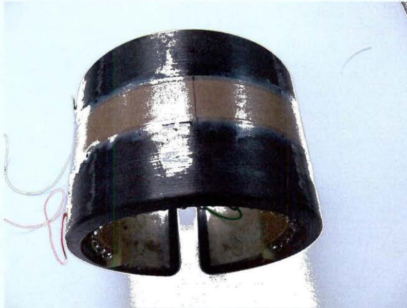
Figure 21 Photograph of an M-25585-P1 MFC bonded to a slotted cylinder transducer
