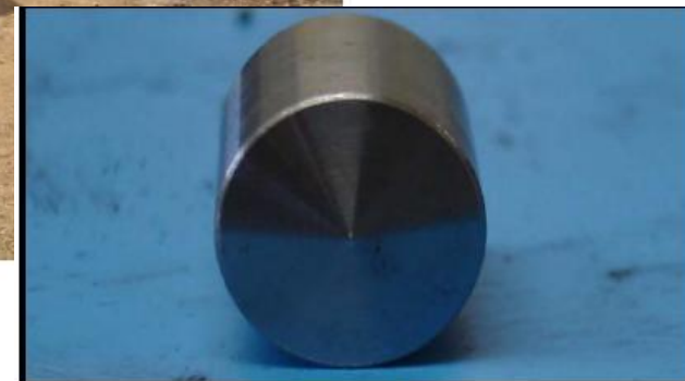
Figure 18 .50-in. mild steel conical army fragment
