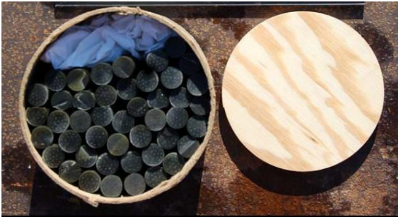
Propellant Sticks loaded in 6 in x 6 in Cardboard Tube
