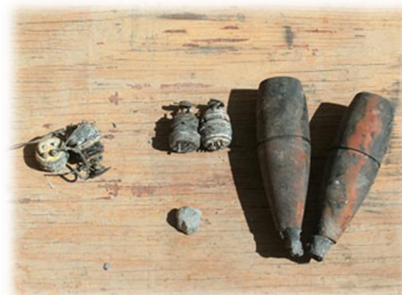
Burned-out 60mm M768 projectiles recovered from MRAP
