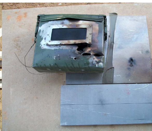
Post Test Results T/S 331-360 / Test 2 Bullet Impact Test
