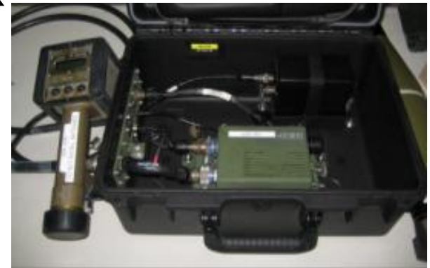
Precision Lightweight Universal Mortar Setter System (XM701 PLUMSS)
