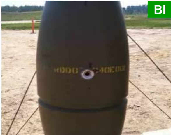
Bullet Impact 81/120mm (TYPE V – 7.62mm)
