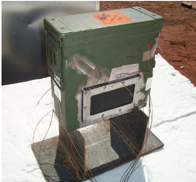
Test Setup T/S 271-300 / Test 2 Slow Cook-Off Test
