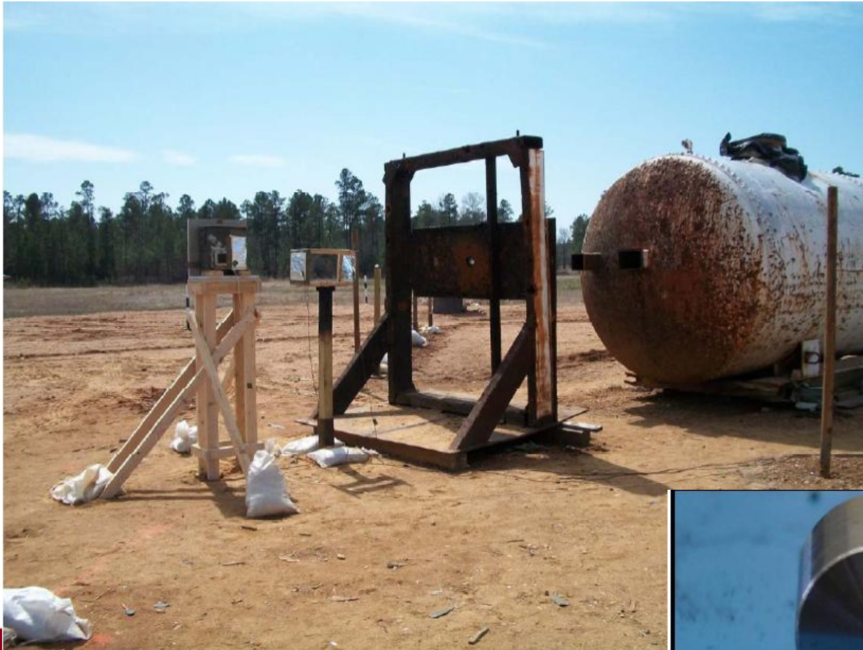
Test Setup T/S 211-240 / Test 2 Fragment Impact Test
