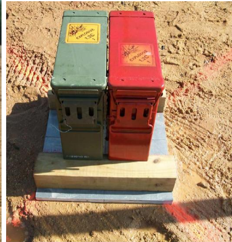
Test Setup T/S 61-120 Unconfined Sympathetic Detonation Test
