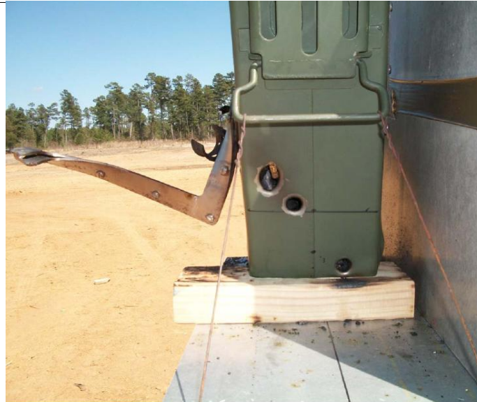
Post Test Results T/S 301-330 / Test 1 Bullet Impact Test
