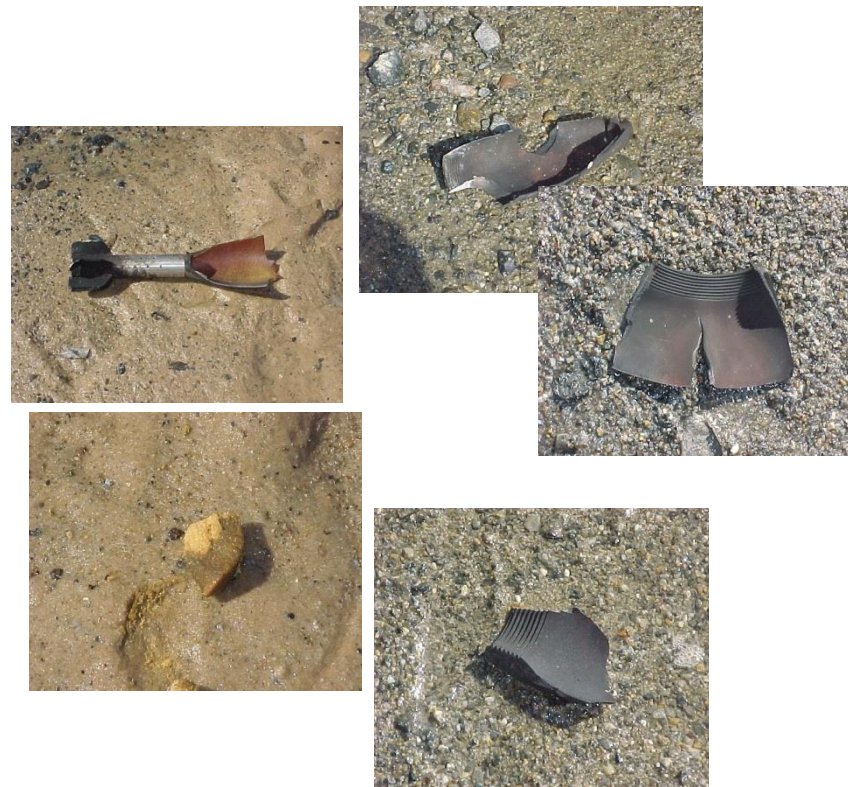
Projectile Body Fragments and Unconsumed COMP B Explosive (TYPE II Response)
