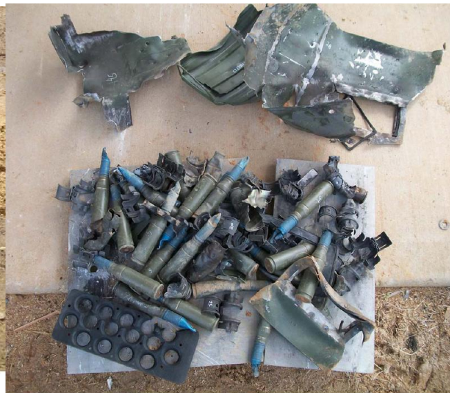
Post Test Results T/S 1-30 / Test 1 Shaped Charge Jet Impact Test
