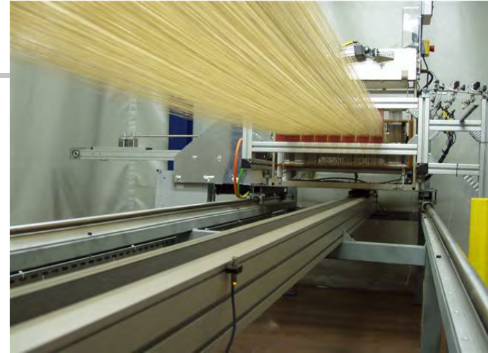
Adaptation of a 24 frames dobby weaving machine for aramid yarns.
