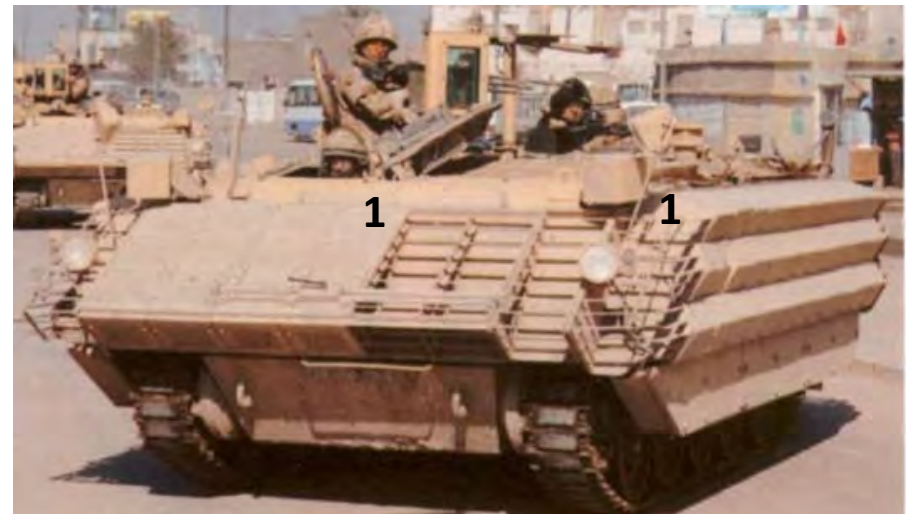
FV432 Mk3 BULLDOG with modular cassettes
