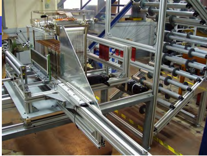
Side view of the automatic multi-layer weaving machine and its specific warp beams creel
