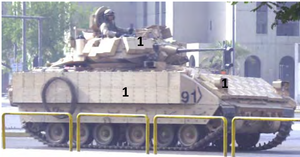
Bradley with different non modular cassettes
