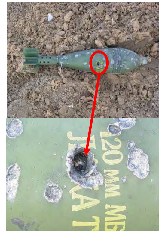
Mortar Arena Test – Fragment Penetration with No Mortar Response
