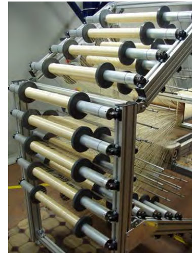
Adaptation of a 24 frames dobby weaving machine for aramid yarns.
