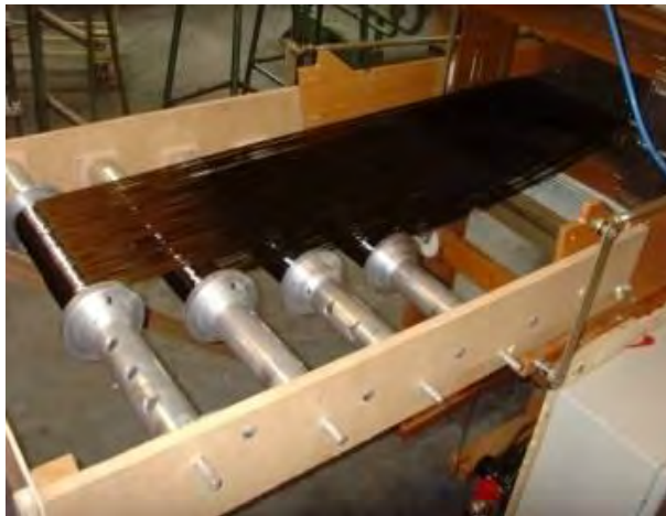
Side view of the automatic multi-layer weaving machine and its specific warp beams creel
