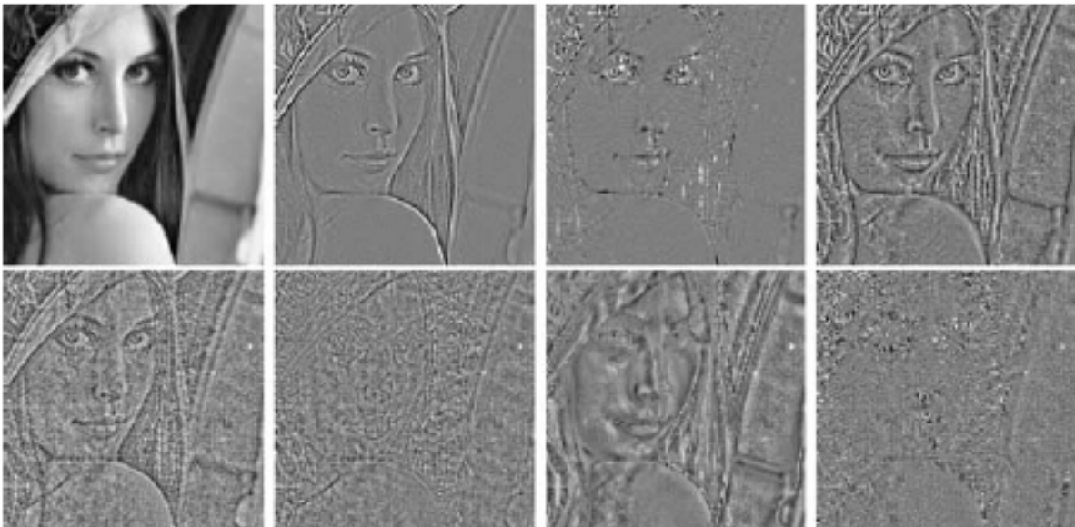
Figure D.2: Method noise experiment on Lena (gray levels only). From top to bottom and left to right: original image, Gaussian mean, mean curvature motion, total variation minimization, translation invariant soft and hard thresholding, bilateral filter and NL-means
