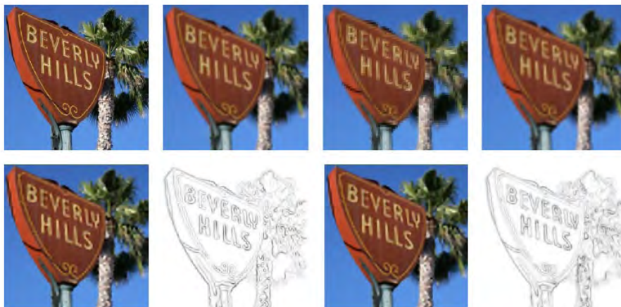
Figure G.3: SUPER-RESOLUTION of a still image. Top: original image of size 272 \times 272 , blurred image h * u with out of focus blur kernel h with radius r = 3 , down-sampled data f = D_k(h * u) of size 68 \times 68 with k = 4 , preprocessed (up-sampled) image \tilde{g} using bicubic interpolation. Bottom: recovered images using (left) MSTV, (right) NL/MSTV.
