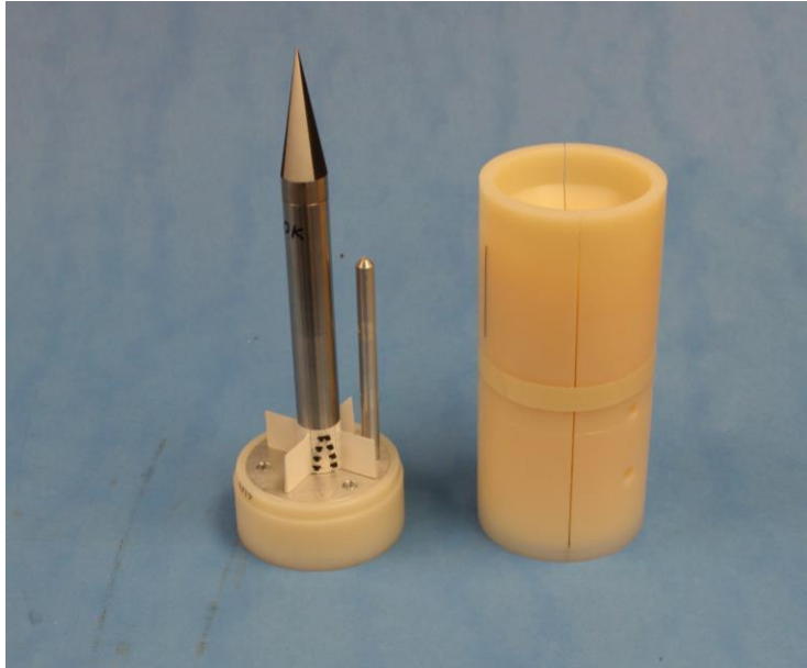
Figure 13. Test Article (active projectile) Used in Outdoor Flight Experiments.
