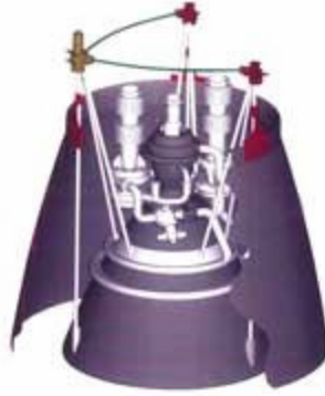
Figure A-1. Extendible Nozzle for Altitude Compensation
