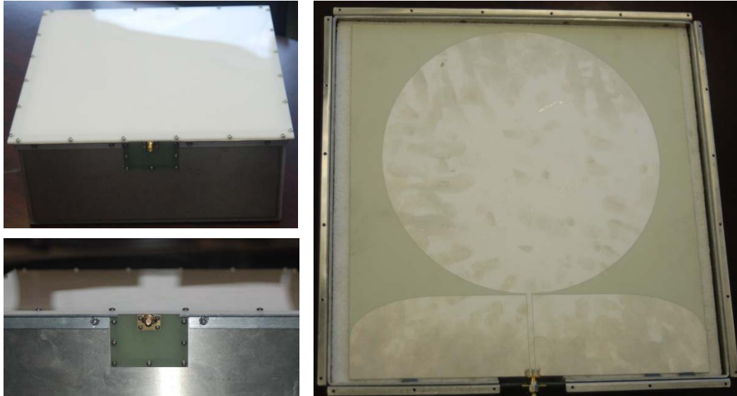
Fig. 16 Completed enclosure (top left), rigidizer (bottom left), and first revision UWB-CPM inside of enclosure (right)
