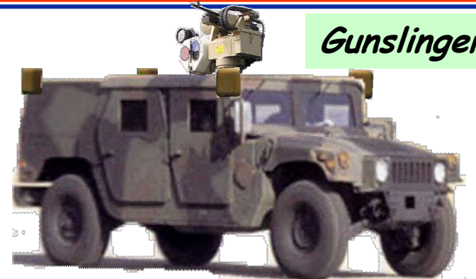
Modular, vehicle based, on-the-move hostile fire detection and counter-fire capability
