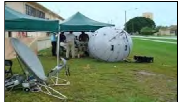
Inflatable satellite antenna, designed to provide high-bandwidth SATCOM capability in a smaller, lighter package than conventional systems
