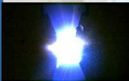
Vaporization of an IHDIV MEMS initiator
