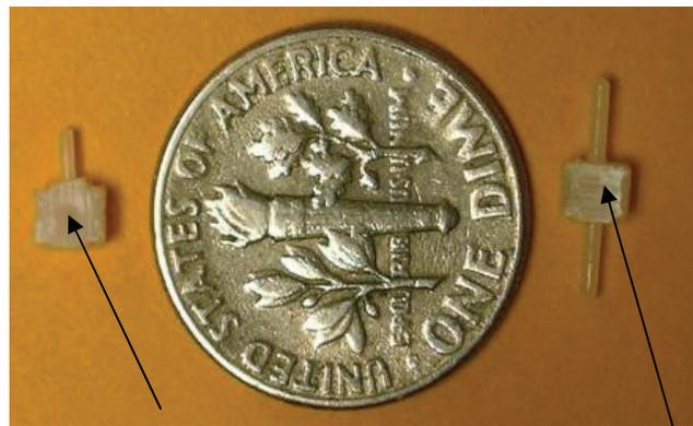
Pin sheared off due to inaccurate core movement
