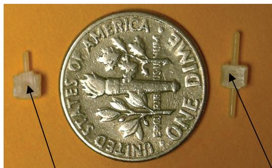
Pin sheared off due to inaccurate core movement      Desirable First stage part
