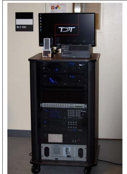
Figure 2 - patient cart. Recordings and stimulation systems, and computers for real-time experimental control and decoding of finger position.
