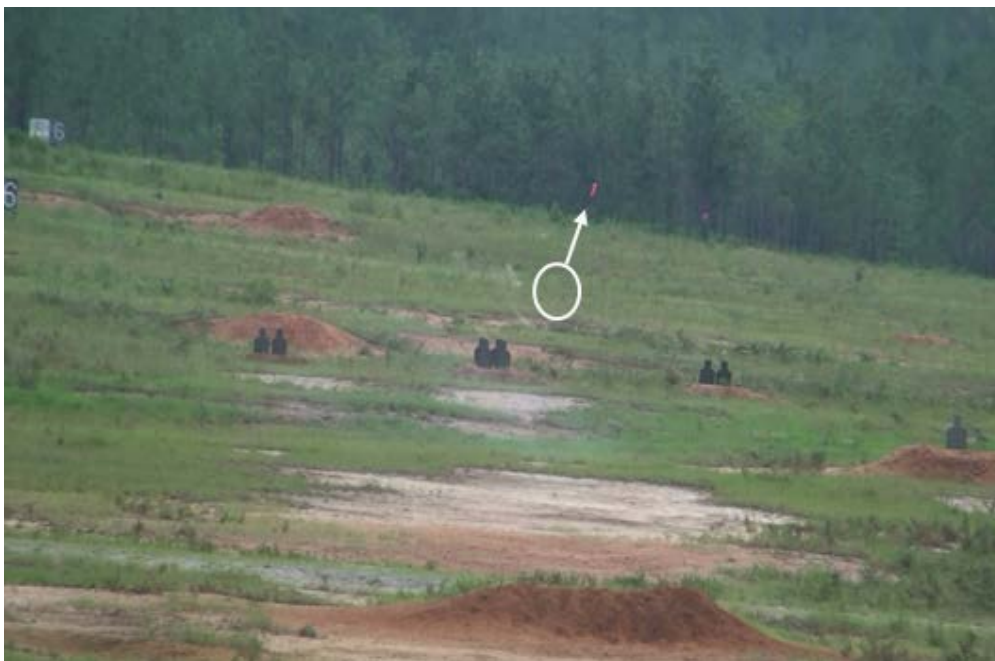
Figure A-2. Path of the same tracer round fired in Fig. A1 that ricochets after hitting the ground near a 600 m target at the Malone 5 range on Fort Benning, GA. Note the upward trajectory of the bullet.
