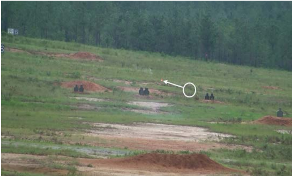
Figure A-1. Initial horizontal trajectory of a tracer bullet fired at a 600 m target at the Malone 5 range on Fort Benning, GA.
