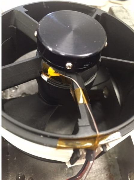
Figure 3.23 Fan Thermocouple Placement
