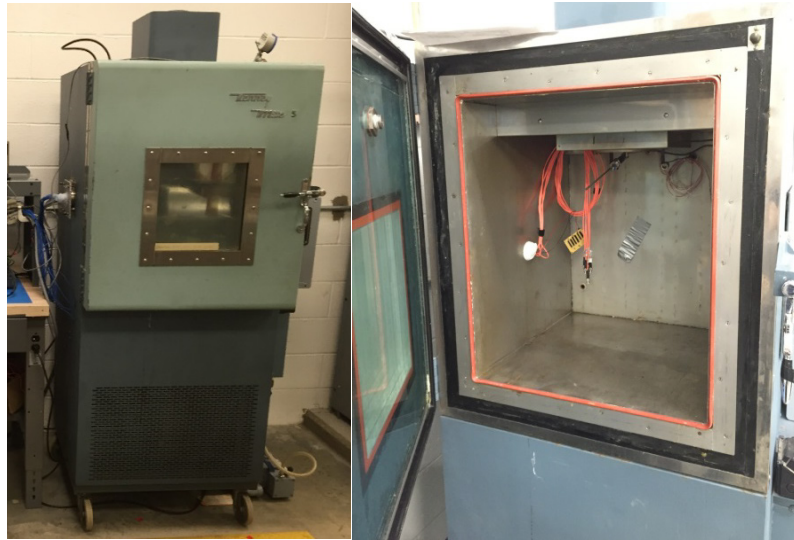
Figure 3.2 Tenney Versa 3 Environmental Chamber (Left) with Working Volume (Right).
