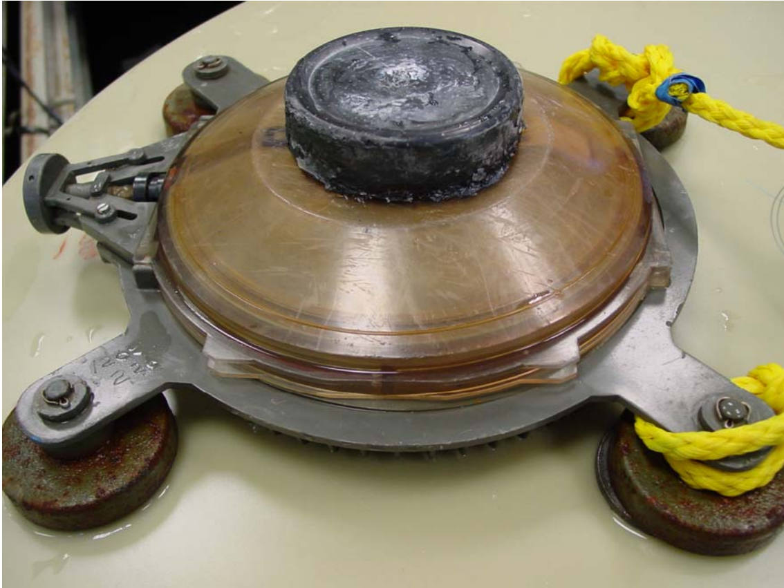
Figure 15 Ball bearing-embedded mineshape atop polymer-bodied practice limpet mine.
