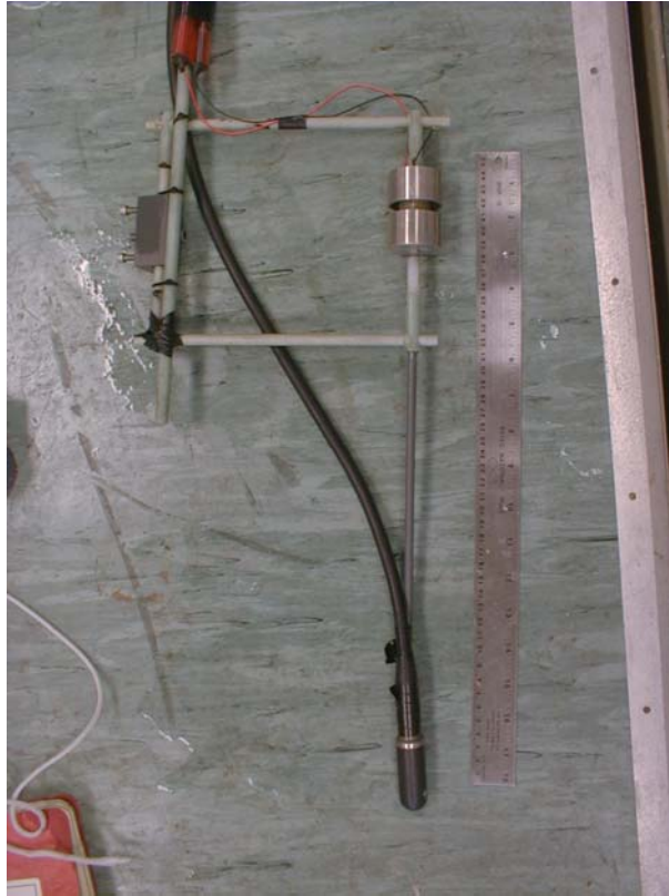
Figure 6 Detail of HF MMPP/hydrophone for first experimental set-up.
