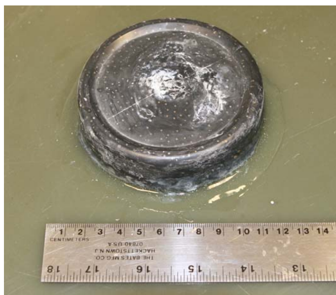
Figure 14 Mineshape with embedded steel ball bearings.
