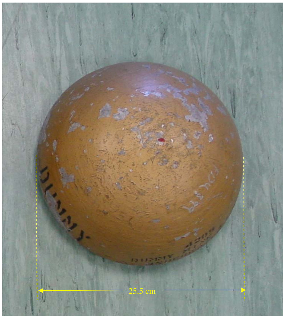
Figure 12 Hemispherical practice limpet mine top-view with dimensions.
