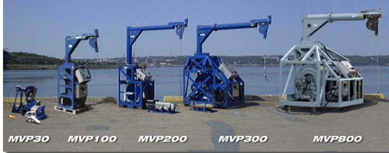
**Figure 1: Moving Vessel Profiler Family of Systems**
