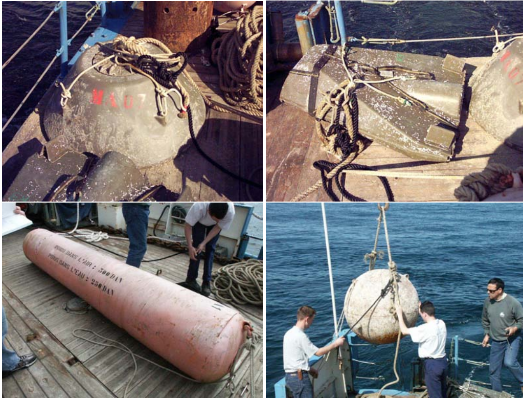
Figure 3: Deployed mine-shaped targets: clockwise from upper left are the Manta, Rockan, sphere and cylinder. (Manta and Rockan photos c/o GESMA.)
