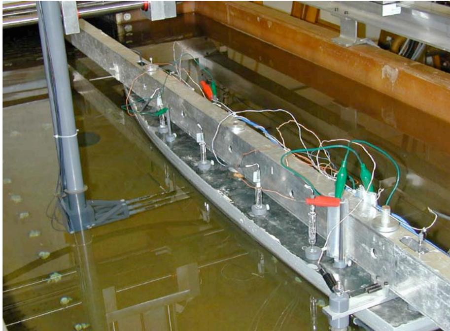
**Figure 14:** A picture of a physical scale model of the Canadian Patrol Frigate developed at DRDC Atlantic to study the underwater electric field signature.
