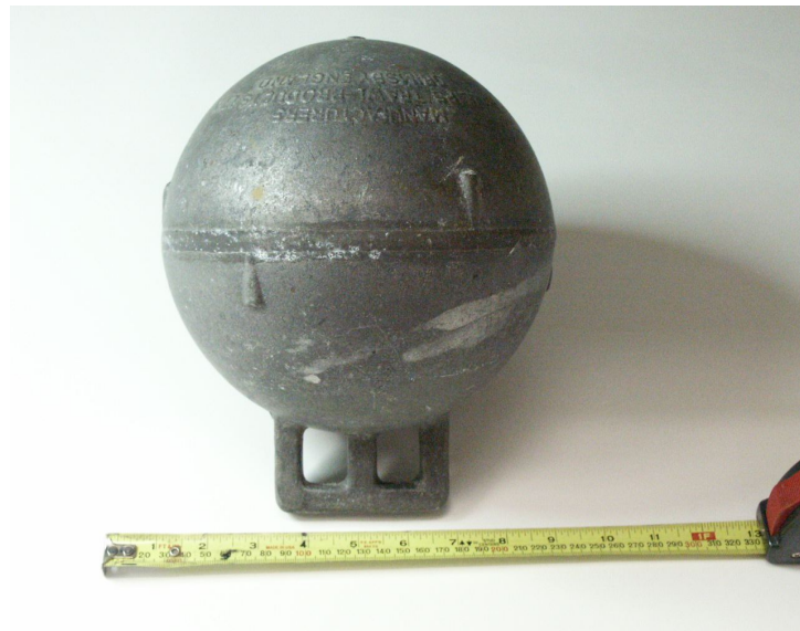
Figure 29: The small aluminum-shelled sphere that was deployed in tank
