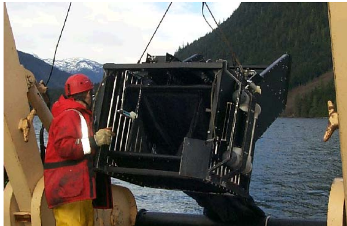
Figure 7 BIONESS multi-net zooplankton trawl ready for deployment. System has 9 remote-controlled nets with 0.25 \text{ m}^2 mouth opening and 0.23 \text{ mm} mesh size.
