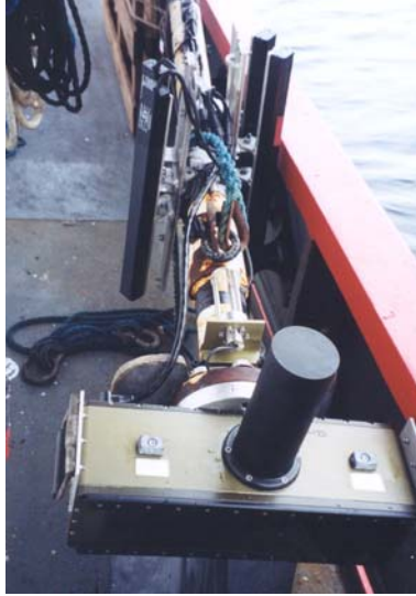
Figure 6 Reson 8125 multibeam sonar mounted on the bottom of a strut mounted on the port side of the CCGS Vector , Nov. 2002. For deployment the strut swings downward to a vertical position with the sonar head at 3.35 m depth.
