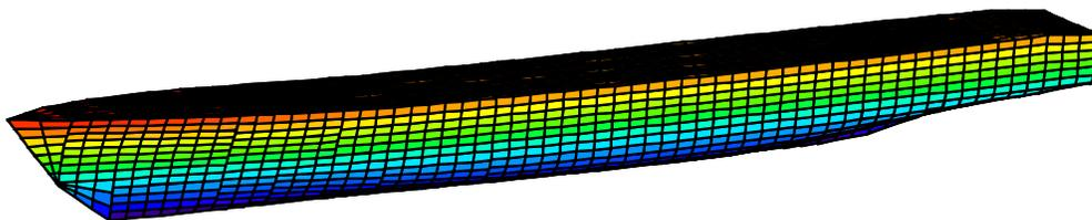
**Figure 8:** *Medium Mesh for Hull of CPF Hydroelastic Model*
